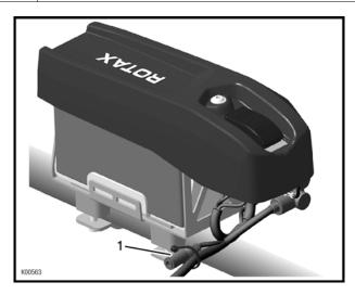
Figure 2.1: Pos. 1: Charging connector
